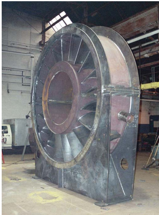
Figure 12: Fan Housing, reassembled with minimal misalignment, awaiting transport to machine shop.
