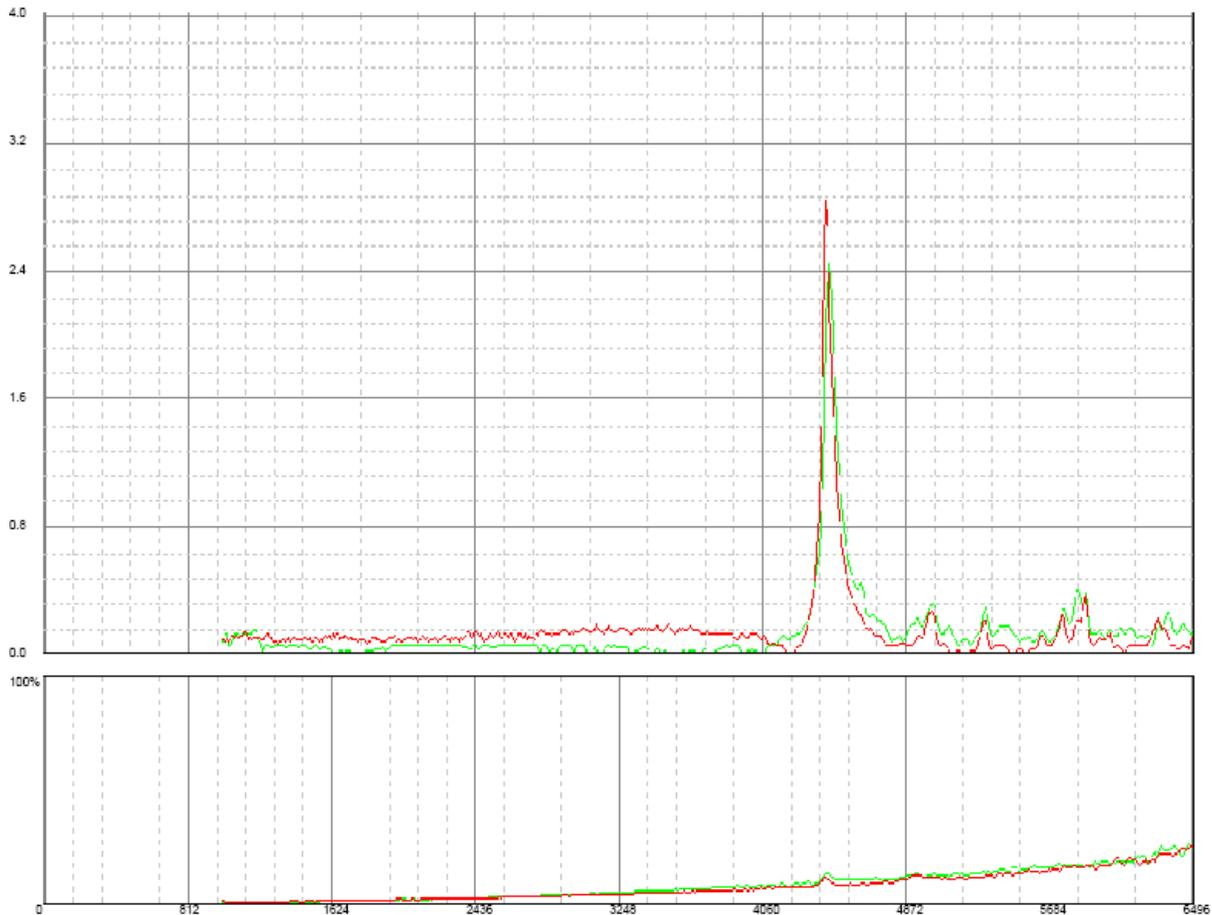
**Figure 4:** Workpiece 1, Treatment 1. The Pre-Treatment Scan plotted in green as shown in Figure 3, with the Post-Treatment Scan, plotted in red, superimposed upon it. Most of the treatment time was spent on the large peak at  $\approx 4500$ -RPM (15-minutes), with each of the peaks to the right of this large peak being tuned upon for 2-3 minutes, to determine if additional peak growth or shifting could be generated. The small peaks yielded little change.
