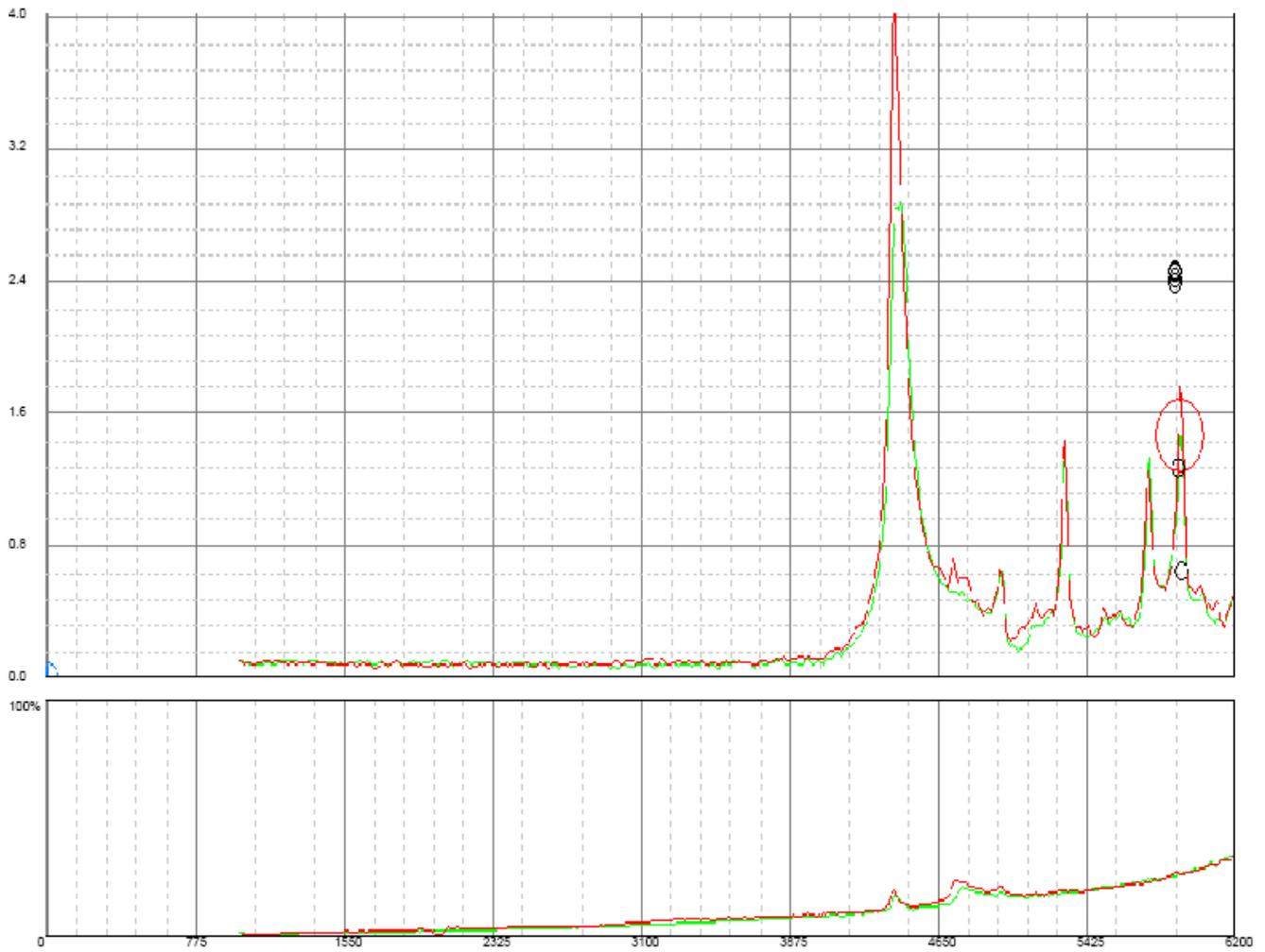
**Figure 9:** Figure 9 shows the 1st VSR Treatment done on Workpiece 3, again we see a significant change in resonance pattern; Figure 10 shows the 2nd Treatment done on Workpiece 3, as expected it displays little resonance pattern change
