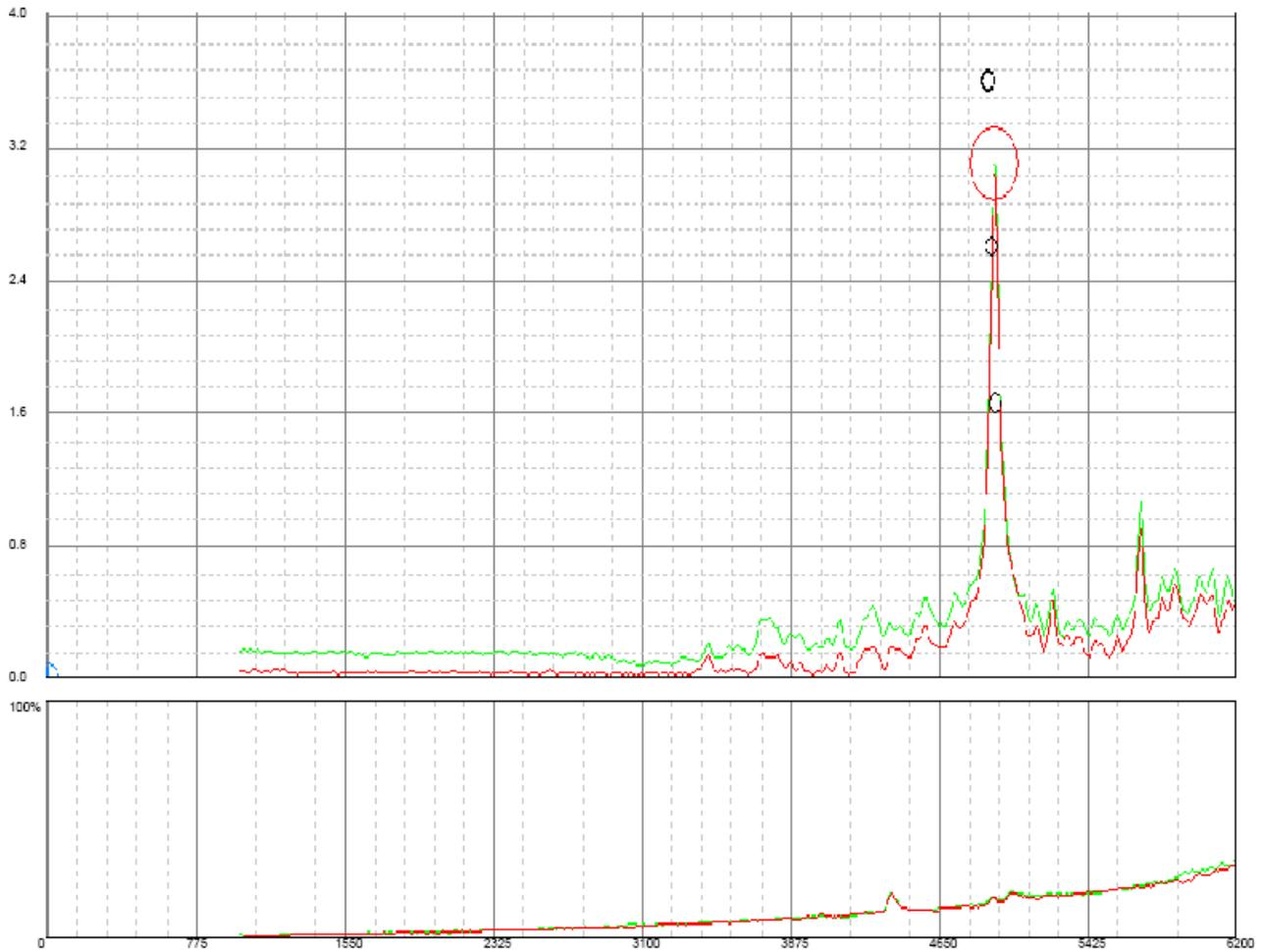
**Figure 8:** (Workpiece 2, 2nd Treatment) shows the second Treatment (using the different Accelerometer location), with very little change in the resonance pattern, which indicates that little additional stress relieving occurred during this Treatment, in all likelihood because Treatment was very effective.
