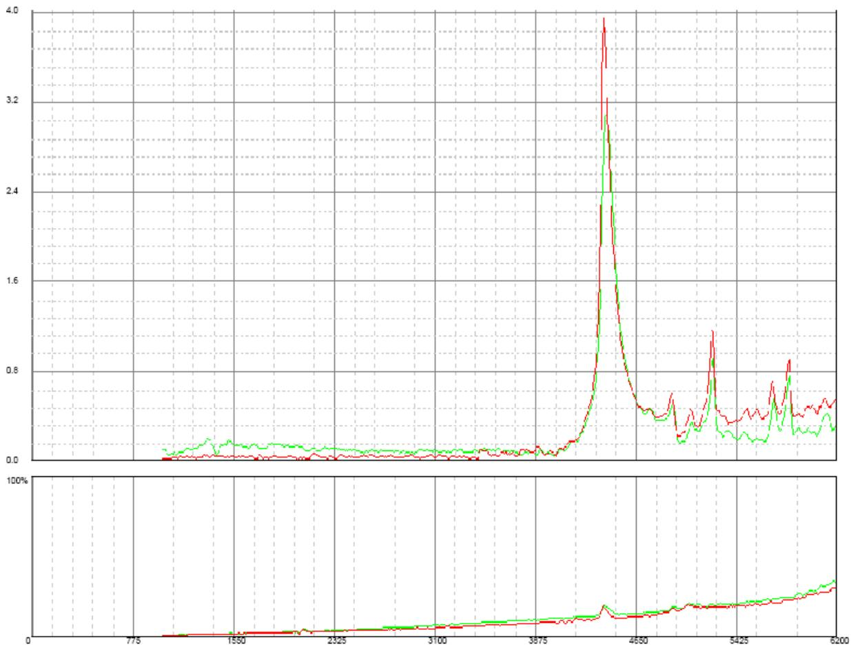
**Figure 7:** Workpiece 2, Treatment 1. Here the growth of  $\approx 20\%$  seen in Workpiece 1 is seen again. Peak growth of this degree is clear indication that these workpieces were dimensionally unstable, but, with VSR Treatment, would now be much more dimensionally stable and predictable.
