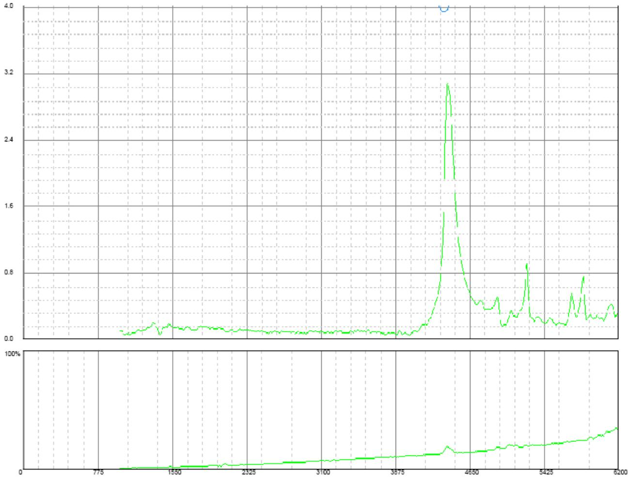
**Figure 6:** Workpiece 2 also received two Treatments, with repositioning and reorienting the Accelerometer the only difference between the Treatments (same as Workpiece 1). Figure 6 shows the Pre-Treatment Scan, and Figure 7 shows the Treatment in progress using this Pre-Treatment Scan. This VSR Treatment displays a growth of 20% in the height of the large resonance peak, about the same as Workpiece 1.
