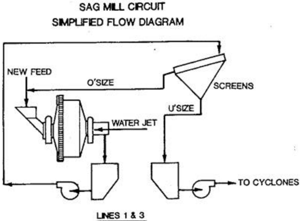
I've got to explain this a little bit. This flowsheet is typical of lines 1 and 3. The SAG mill has a trommel on the discharge end of it. Oversize is returned to the mill by a bucket wheel and water jet. Trommel undersize was pumped to a vibrating screen where the screen oversize was sent back to the mill and the undersize was pumped to the cyclone circuit. Figure 2 shows the flowsheet for line 2 with only the trommel,
