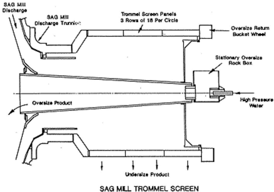
The next two photographs show the trommel prior to startup before the cover and the stationary rock box were installed. The bucket wheel and the urethane panels can be clearly seen. Screen panel size is 28 by 54 inches. The oversize return tube turns with the trommel
